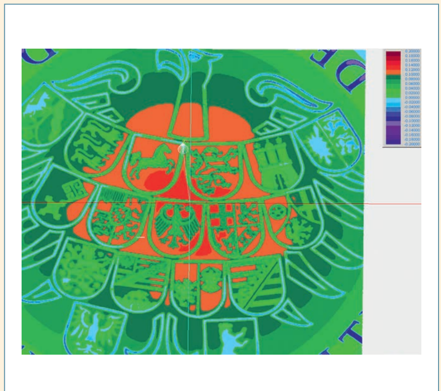
Figure 1. Scanning an embossing die for coins along a defined path without feedback control, using an optical distance sensor (color-coded deviation from a best-fit plane, as the model was understandably not available)
