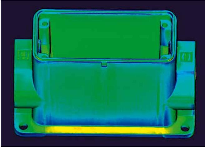
▲ Deviation analysis: The CAD model is merged or „Best Fit“ with the tomographically captured data and deviations are plotted in color.
