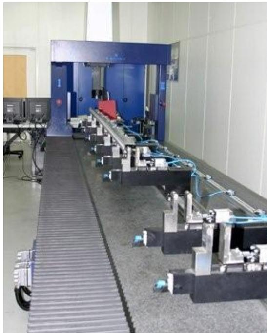
**For PFW Aerospace, Werth Messtechnik expanded the Werth ScopeCheck MB, a 3D CNC multi-sensor coordinate measuring machine, with a six meter long, 13 ton granite table**
