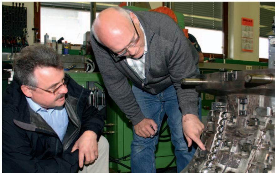
**Correction.** Herbert Layher (left, HeMa CT) and Werner Vesper (Vema) inspect the molds, which are the foundation of high-precision plastic components. After measuring the first injection molded parts, one or more corrections must be made to the mold to optimize the precision of the parts..
