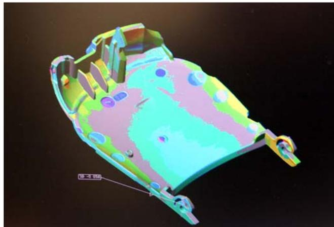
**Figure 3. Data for a sample part, captured by the coordinate measuring machine, are read into the software, along with the CAD data of the nominal part. The deviations between the actual and nominal data are displayed graphically.**
