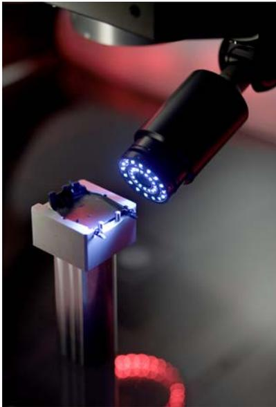
until now. Multisensor machines from Werth Messtechnik GmbH, Giessen, Germany, solve this problem with optical, tactile, and laser technologies. A special optical sensor head, mounted on a rotary/tilting adapter joint, allows the optics to measure from several directions.
