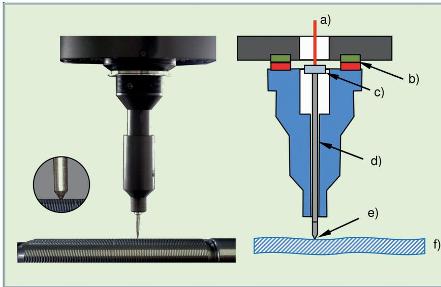
Figure 2. Werth Contour Probe (WCP): additional equipment for tactile contour measurement with distance sensors: a) Measurement beam, b) Magnetic interface, c) Mirror, d) Guide, e) Probe tip, f) Workpiece
