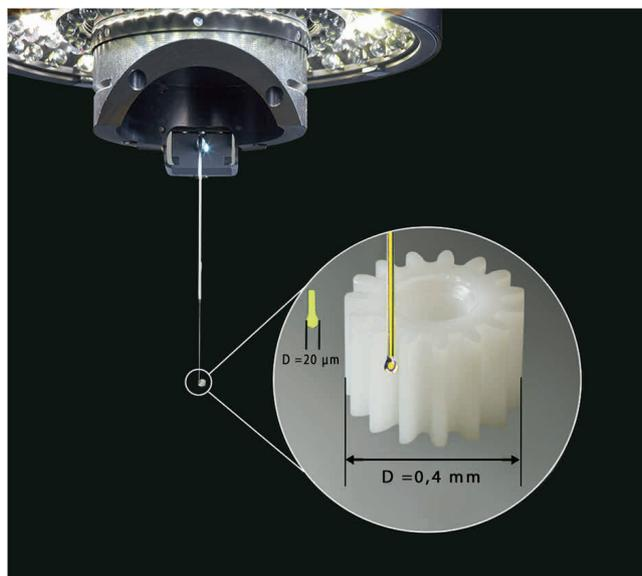
Figure 1: Measurement of a micro gear with the Werth Fiber Probe – the fiber is guided in a metal tube. (© Werth)
