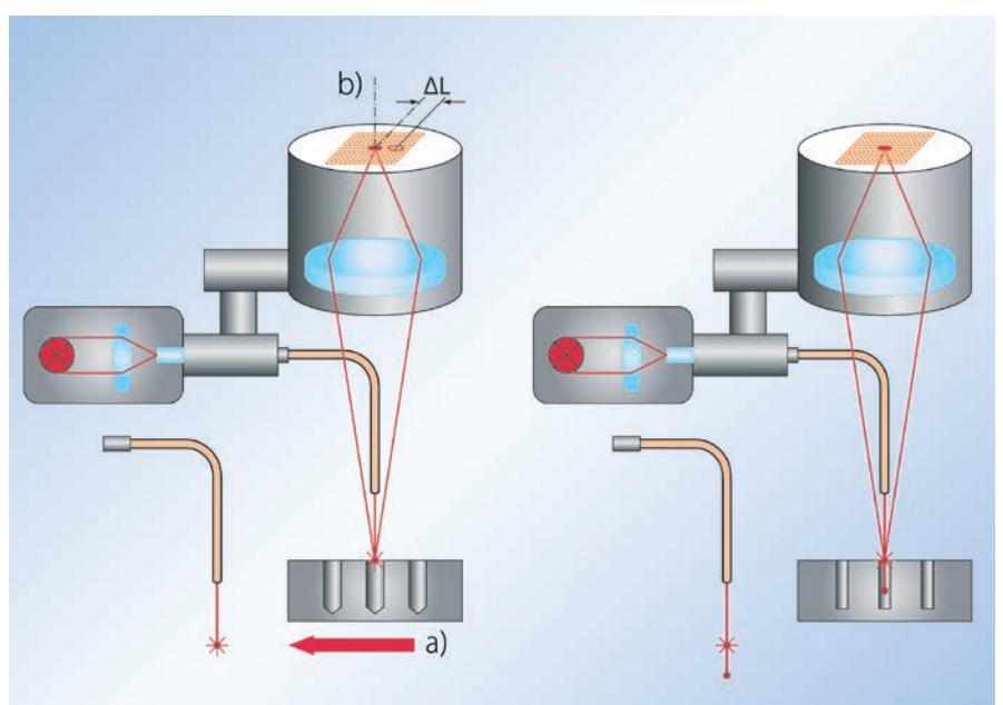
**Figure 1.** Functional principle of the fiber probe: Single-sphere probe (left): movement of the measured object (a) causes contact and deflection  $\Delta L$  from the sensor origin in the image plane of the camera (b). Dual-sphere probe (right): even when contact is made at a great depth, the sphere is not in the shadow of the object.
