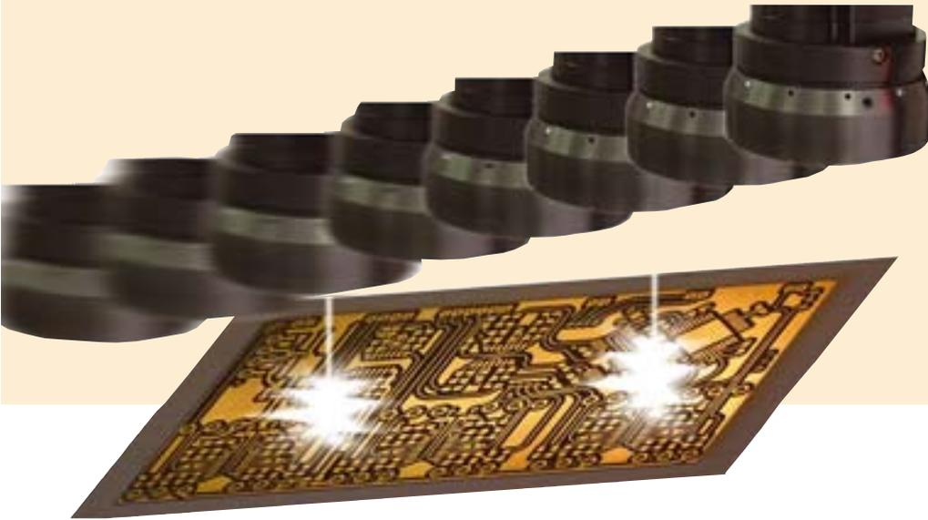
*Fig. 1 OnTheFly – Highly advanced control technology enables the measuring machine to measure features precisely while in motion.*
