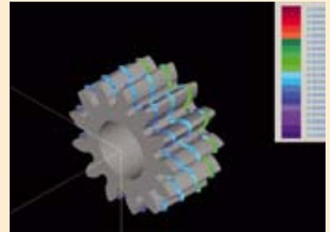
Fig. 3 Profile deviation of a microgear scanned with the Werth Fiber Probe
