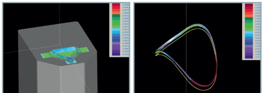
1 Color-coded presentation of deviations on different workpieces, measured using various sensors:
