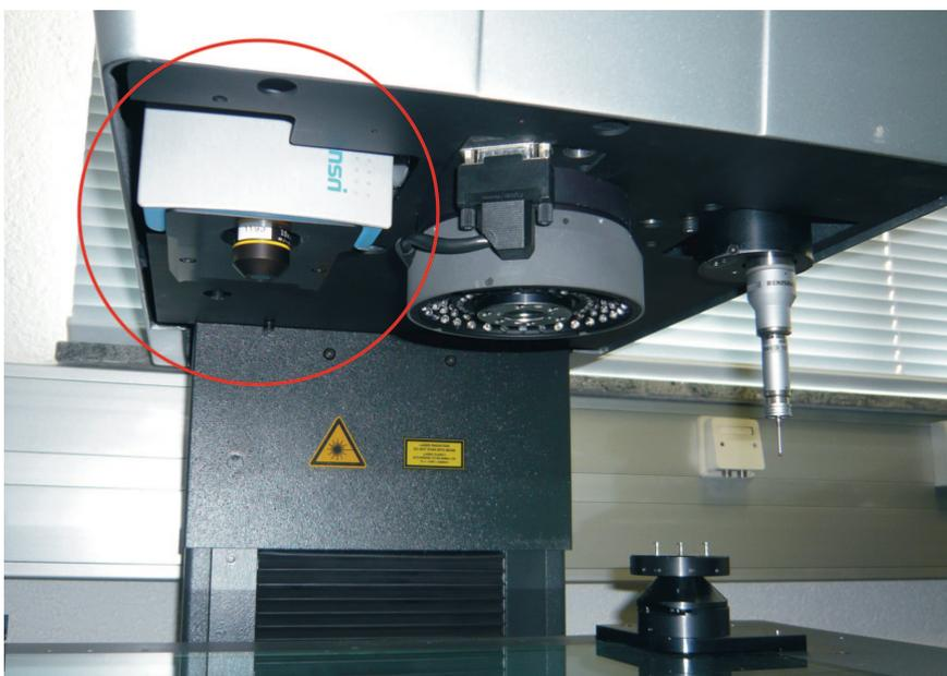
3 Werth ›VideoCheck 400x200x200‹ with integrated NanoFocus sensor
