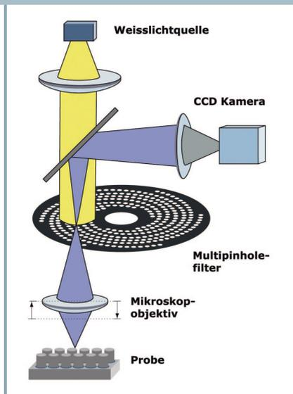
4 Functional principle of the NanoFocusProbe
