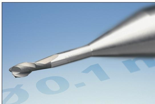
Figure 1. Complete machining, using HSC high performance mills to obtain the final shape, is possible only with form cutter tolerances of  $\pm 2 \mu\text{m}$  and runout of less than  $2 \mu\text{m}$ . Image: Zecha
