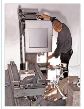
A look at the sensors, not yet "hidden" behind thick lead plates, on the new Werth TomoScope\* HV 500
