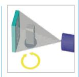
The measured object is rotated 360° for complete X-ray capture
