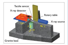
Mechanical construction of the Werth TomoScope®
