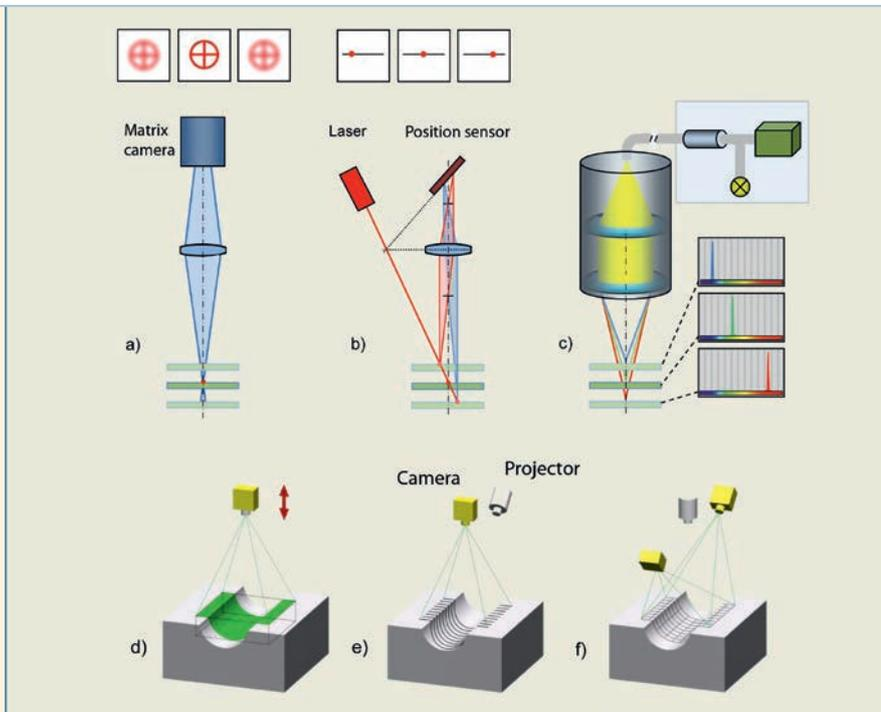
**Figure 2. Overview of optical distance sensors. Pointwise distance measurement sensors:**
