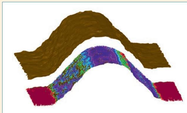
**Figure 1. High-resolution area measurement with 3D Patch: Meshed view of the measured surface (top), color-coded deviation plot to the CAD model (bottom)**
