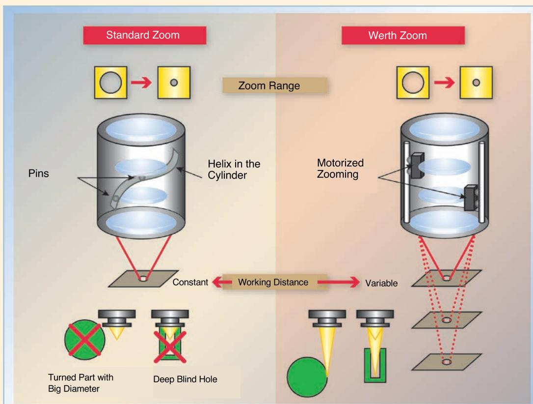
Figure 1. Zoom with helical control slots in the lens barrel (left), Werth Zoom with motorized linear guides and variable working distance (right)
