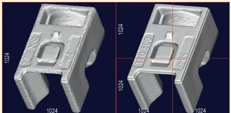
Figure 1. Point clouds (STL view) measured using tomography at low resolution (left) and using raster tomography at high resolution (right)
