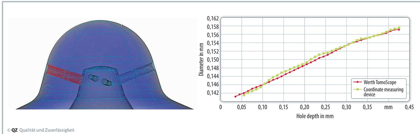
Fig. 2. Comparison measurement of the diameter of a fuel injection nozzle with computed tomography and high-precision fiber probe (a); display of measured volume and measuring point cloud in the area of the spray. (© Werth Messtechnik)
