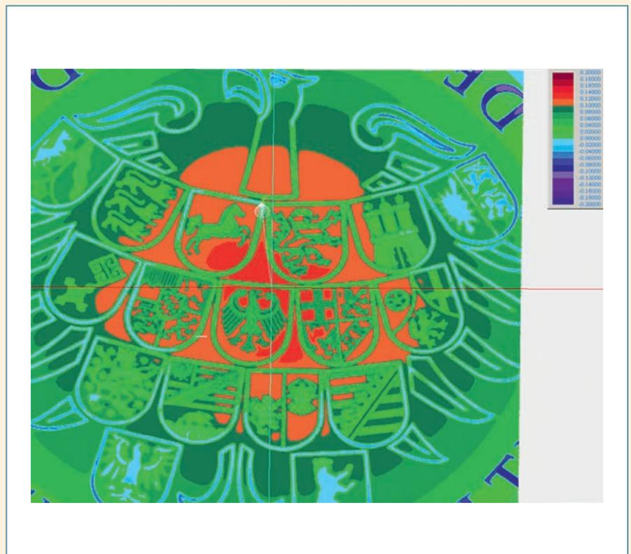
Figure 1. Scanning an embossing die for coins along a defined path without feedback control, using an optical distance sensor (color-coded deviation from a best-fit plane, as the model was understandably not available)
