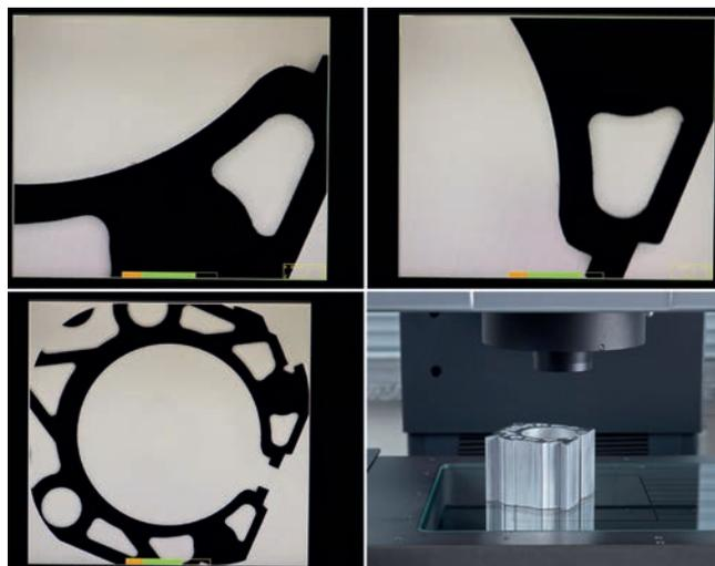
Figure 2. Tracing the workpiece edge with raster scanning using the image processing sensor (© Werth)
