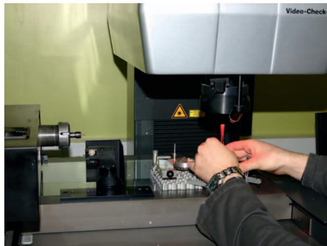
Figure 3. The measurement area was designed such that clamps and most fixtures can remain on the machine, which allows faster changeover of parts.
